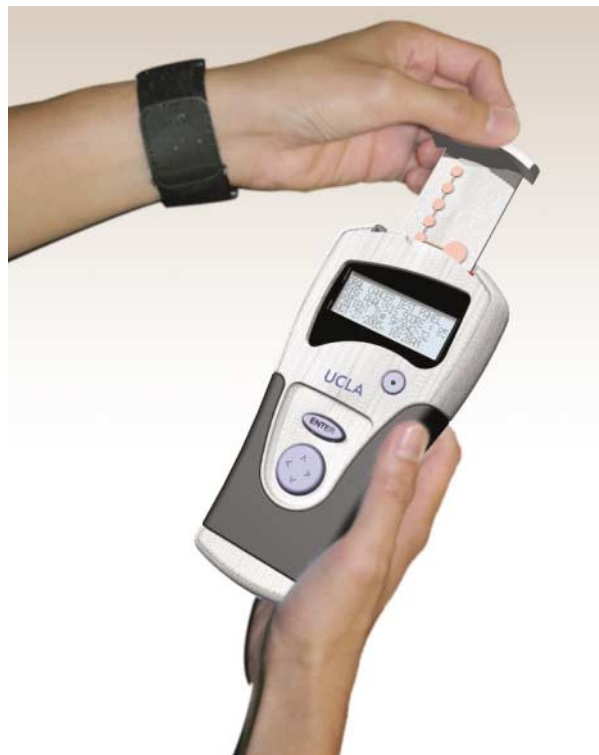
Figure 4. Oral Fluid NanoSensor Test, a handheld, automated, easy-to-use integrated system that will enable simultaneous and rapid detection of multiple salivary protein and nucleic acid targets.
